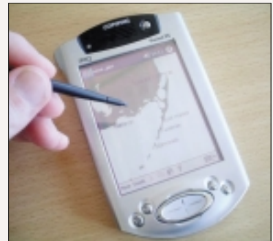
RaveGeo is a fast, compressed, multi-resolution format for huge geographic vector databases, designed for environments ranging from handheld devices to desktop applications
